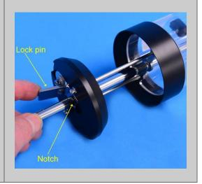
The water sampler is now loaded, ready for deployment.
